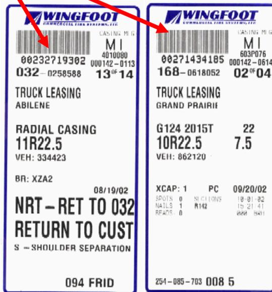
All casings brought into retread production system are tagged – the tag is affixed to tire, to Plant Work order, and is part of finished tire label
